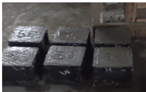
Figure 5 cubes of concrete replaced with coconut and sea shells aggregate
